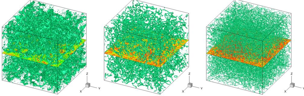
Figure 20: RVR-QT. Instantaneous fields computed with the real-time GP solver, starting from the initial condition presented in Fig. 19. Vortex lines (iso-surfaces of low  $\rho$ ) of the wave function at final time  $T_f$ . From left to right: grid resolutions  $N_x = 128, 256, 512$  (corresponding to runs RVR\_a, RVR\_b and RVR\_c in Table 12).
