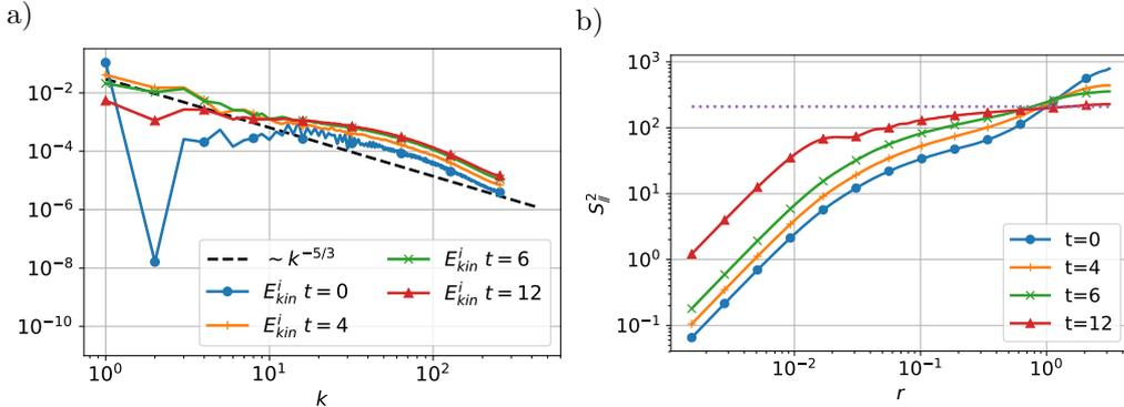
Figure 7: TG QT. Spectrum of  $E_{kin}^i$  (a) and second-order structure function (b) for the case TG\_c (see Table 2).
