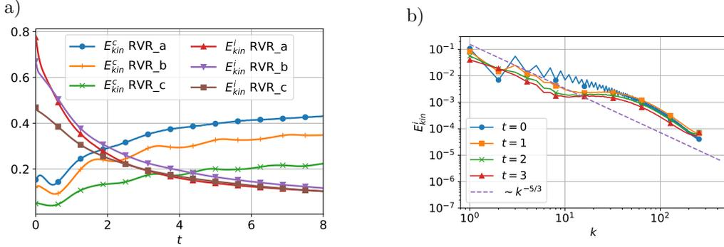
Figure 21: RVR-QT. (a) Time evolution of the compressible  $E_{kin}^c$  and incompressible  $E_{kin}^i$  kinetic energies. (b) Spectrum of  $E_{kin}^i$  at different time instants. Case RVR\_c ( $N_x = 512$ ). In both panels, the results represent an ensemble average for 10 different runs, with random initial distribution of  $N_V = 800$  vortex ring pairs in the computational domain.
