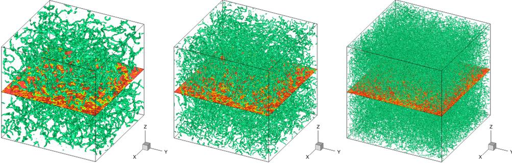
Figure 11: ABC-QT. Instantaneous fields computed with the real-time GP solver, starting from the initial condition presented in Fig. 9. Vortex lines (iso-surfaces of low  $\rho$ ) of the wave function at final time  $T_f$ . From left to right: grid resolutions  $N_x = 128, 256, 512$  (corresponding to runs ABC\_a, ABC\_b and ABC\_c in Table 7).
