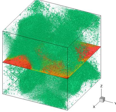
Figure 17: SRP-QT. Instantaneous fields computed with the real-time GP solver, starting from the initial condition presented in Fig. 2. Vortex structures (iso-surfaces of low  $\rho$ ) of the wave function at final time  $T_f$ . Grid resolution  $N_x = 512$ , corresponding to run SRP\_c in Table 11).
