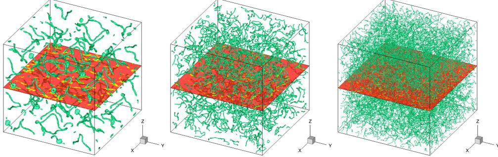
Figure 5: TG-QT. Instantaneous fields computed with the real-time GP solver, starting from the initial condition presented in Fig. 4. Vortex lines (iso-surfaces of low  $\rho$ ) of the wave function at final time  $T_f$ . From left to right: grid resolutions  $N_x = 128, 256, 512$  (corresponding to runs TG\_a, TG\_b and TG\_c in Table 2).
