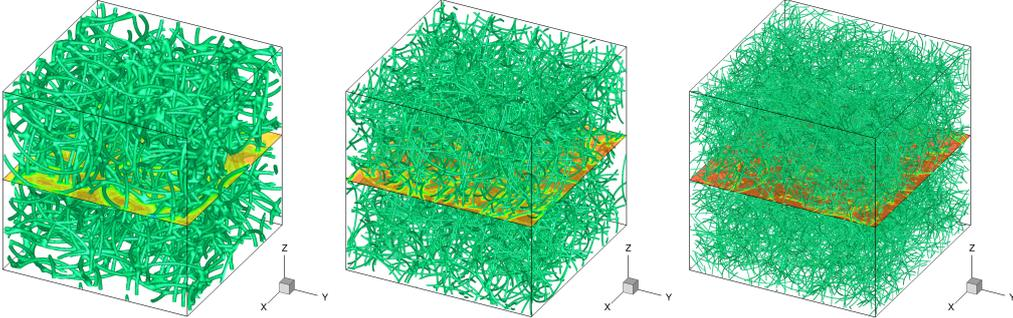
Figure 19: RVR-QT. Initial field containing  $N_V$  randomly distributed vortex ring pairs. Vortex lines (iso-surfaces of low  $\rho$ ) of the wave function. From left to right: grid resolutions  $N_x = 128, 256, 512$  and  $N_V = 200, 400, 800$  (corresponding to runs RVR.a, RVR.b and RVR.c in Table 12).
