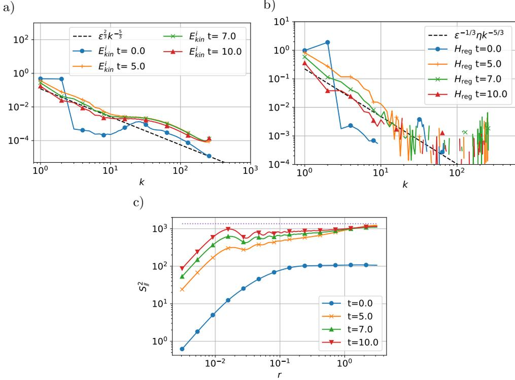
Figure 13: ABC-QT. Analysis of the turbulent super-flow. Spectrum of incompressible kinetic energy  $E_{kin}^i$  (a) and regularized helicity  $H_{reg}$  (b) at different time instants for case ABC.c. Dashed lines represent reference power laws with slope  $-5/3$ . Panel (c) displays the second order structure function for the same case ABC.c and same time instants.
