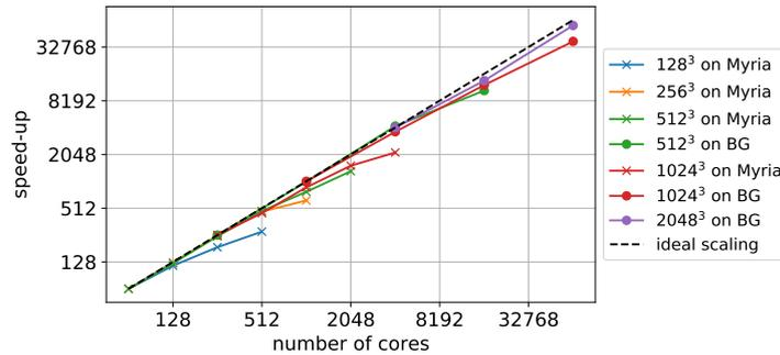
Figure A.22: Parallel performance (speed-up) of the GPS code when computing 3D cases with  $128^3$ ,  $256^3$ ,  $512^3$ ,  $1024^3$  and  $2048^3$  grid points. Strong scalability test using only MPI (from 64 to 64,536) processes. Dashed lines represent ideal speed-up.
