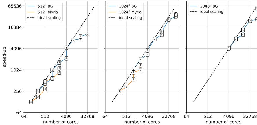
Figure A.23: Parallel performance (speed-up) of the GPS code when computing 3D cases with  $512^3$ ,  $1024^3$  and  $2048^3$  grid points. Strong scalability test of the hybrid code MPI-OpenMP using MPI processes as in the previous test and 1, 2 or 4 OpenMP threads. Dashed lines represent ideal speed-up.
