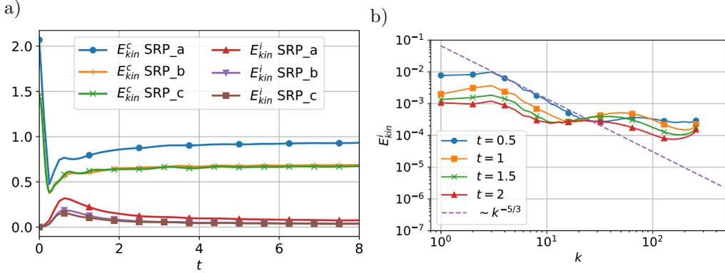
Figure 18: SRP-QT. (a) Time evolution of the compressible  $E_{kin}^c$  and incompressible  $E_{kin}^i$  kinetic energies. (b) Spectrum of  $E_{kin}^i$  at different time instants. Case SRP\_c ( $N_x = 512$ ). In both panels, the results represent an ensemble average for 10 different (random) initial conditions.
